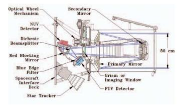
FIG. 1.— A cross section of the instrument portion of GALEX. The optical path is outlined in blue. Overall dimensions of the view shown are  $1.5 \times 1$  m. Solar panels and a separate compartment for spacecraft bus electronics (supplied by Orbital) are not included.
