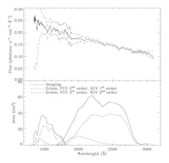
FIG. 3.— *Upper panel:* (Solid line) A composite of 42 ~240 s GALEX spectra of the *HST* white dwarf standard star BD+33°2642. (Dotted line) The *HST* reference spectrum. (Dashed lines) The range of 1 $\sigma$  variations among the 42 spectra. *Lower panel:* (Solid lines) The ground-measured imaging-mode effective area. (Dashed lines) The flight-measured grism-mode effective area. (Dot-Dashed lines) The additional effective area in the grism 2nd (NUV) and 3rd (FUV) orders.
