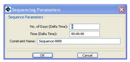
Figure 16.4. The dialogue for creating a Sequence constraint, an ordered interruptible group. This is opened from the Add Sequencing button in the constraint editor dialogue.
