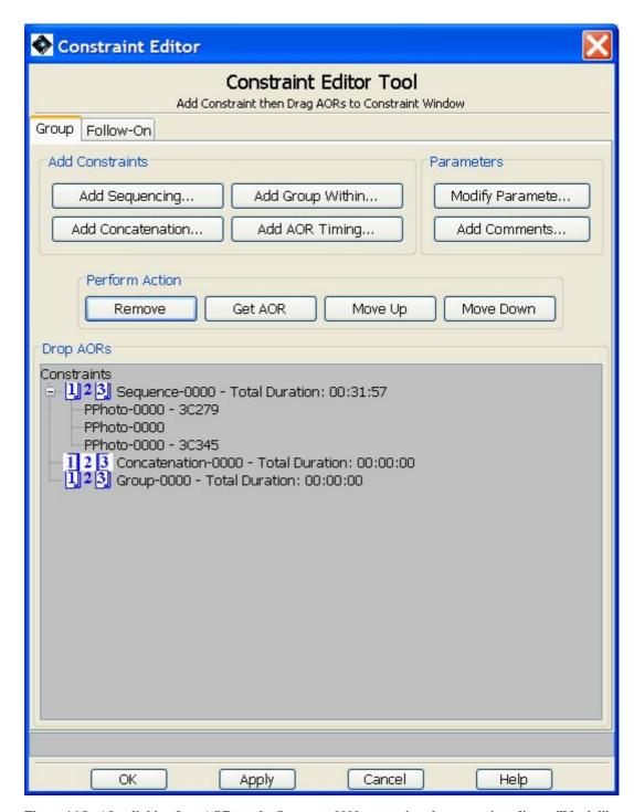
Figure 16.8. After linking four AORs to the Sequence-0000 constraint, the constraint editor will look like this. You can manipulate the order of the AORs by selecting one and using the "Perform Action" buttons to remove the AOR, or to move it up or down in the order.
