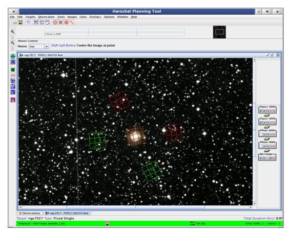
Figure 19.27. PACS Line Spectroscopy "Mapping" observation is shown overlaid on a DSS background image of NGC7027. The chopper off-positions are shown in red. The two footprints correspond to the beginning and end of the object visibility window.
