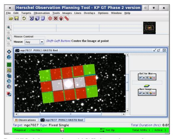
Figure 19.32. Depth of coverage overlay example in PACS point-source photometry mode
