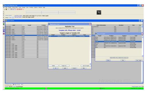
Figure 15.1. An example of replicating an AOR. A PACS photometry AOR has been selected, highlighting it in blue in the observations table. Target 3C345 is then selected from the Target List and dragged and dropped into the Replication Tool window.
