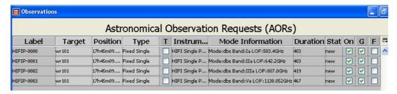
Figure 16.9. AOR listing in the observations table showing the ticked grouping checkbox in the "G" column for AORs in our group constraint.
