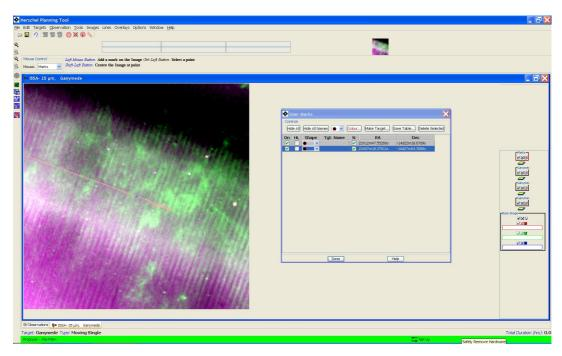
Figure 20.6. Adding marks to an image. Another layer called "Marks" is added to the frame. Clicking on the small red line icon under "Marks" will bring up the dialogue box of "User Marks".
