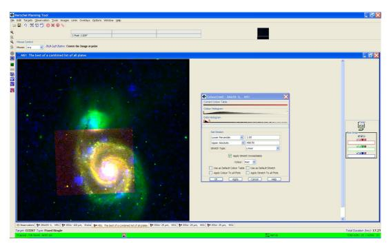
Figure 19.10. An example of changing the data stretch by selecting and dragging one of the red brackets on the data histogram scale. The image display is changed to the values that you have selected and the "Set stretch" changed to "Lower Absolute" or "Upper Absolute" as appropriate.
