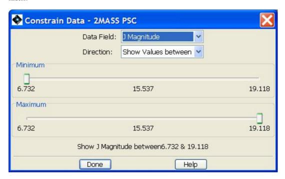
Figure 19.20. Clicking on the "constrain data" icon to the right of the cluster of overlay control icons in the sidebar brings up this dialogue. The dialogue permits the user to change the band and the limiting magnitude/flux of the sources overlaid.
