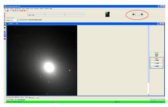
Figure 19.5. The image display icon (circled in red) that allows you to blink between several images in the same frame.
