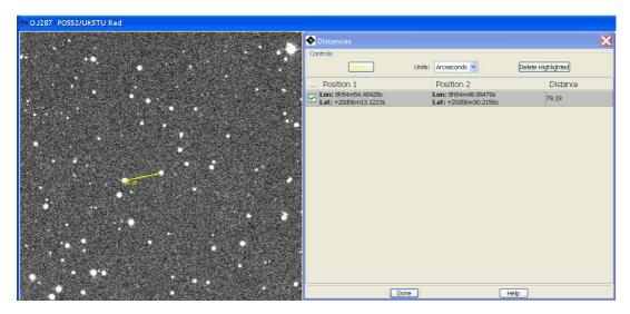
Figure 20.7. The Distance Tool in action. The yellow line indicates the distance between the two selected points. The distance, in arcseconds, is displayed on the image. Detailed information can be brought up in the "Distance" dialogue box.
