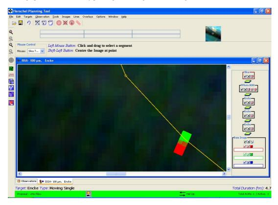
Figure 20.20. When you overlay AORs on an image for a moving target, additional icons appear that allow you to calculate the background across a slice of the image.
