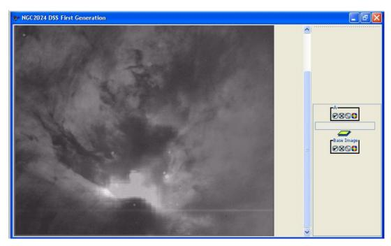
Figure 19.21. An example of Image Overlays. Here we have overlaid a MSX 8.28 micron image on a DSS image of NGC 2024. The opacity of each image can be adjusted using the opacity control. In this example, each image's opacity has been adjusted to 50%.
