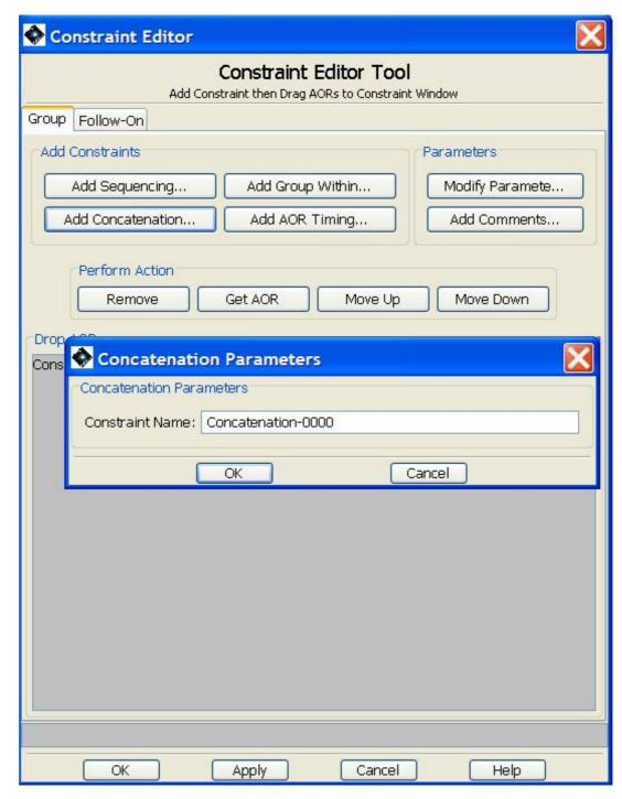
Figure 16.11. The Constraint Editor Tool is then opened and "add Concatanation..." is selected.
