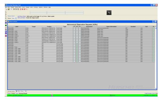
Figure 16.15. The AOR main window when all six concatenations have been defined. All the AORs are flagged in the "G" (Group) column to show that a grouping constraint has been applied.
