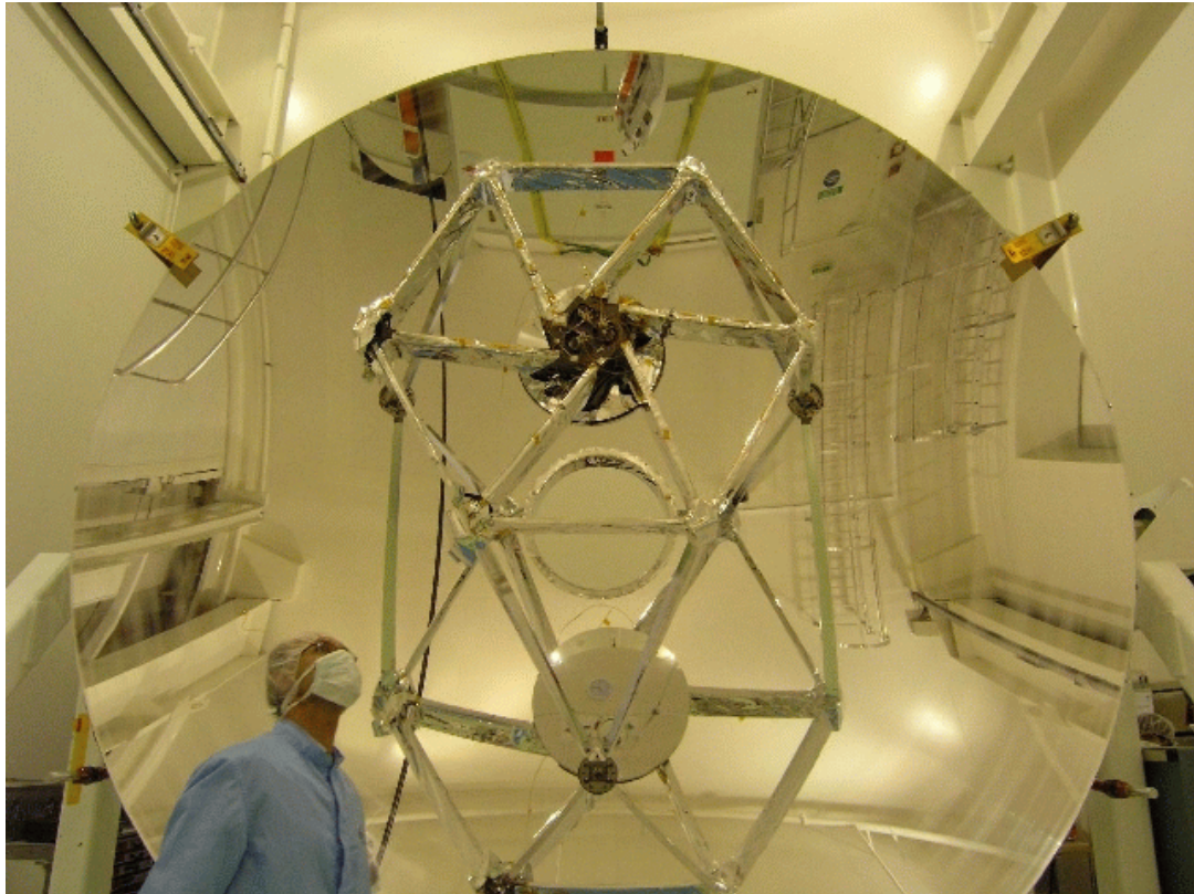
Figure 1.2. The Herschel telescope flight model.
