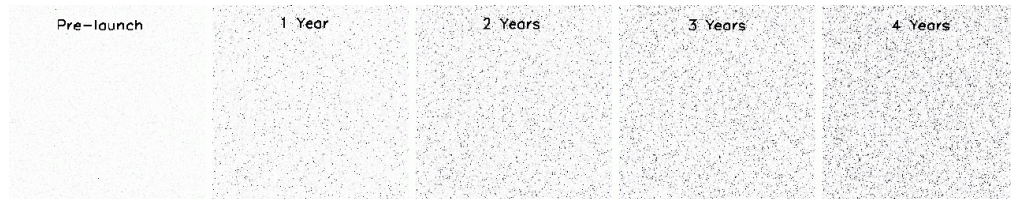
Figure 4.10: A subsection of WFC1 dark frames taken at different epochs showing the increasing population of hot pixels.
