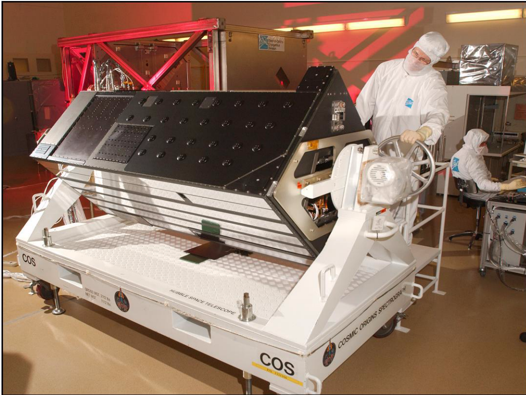
Figure 3.9: The COS flight instrument in its test stand at Ball Aerospace.
