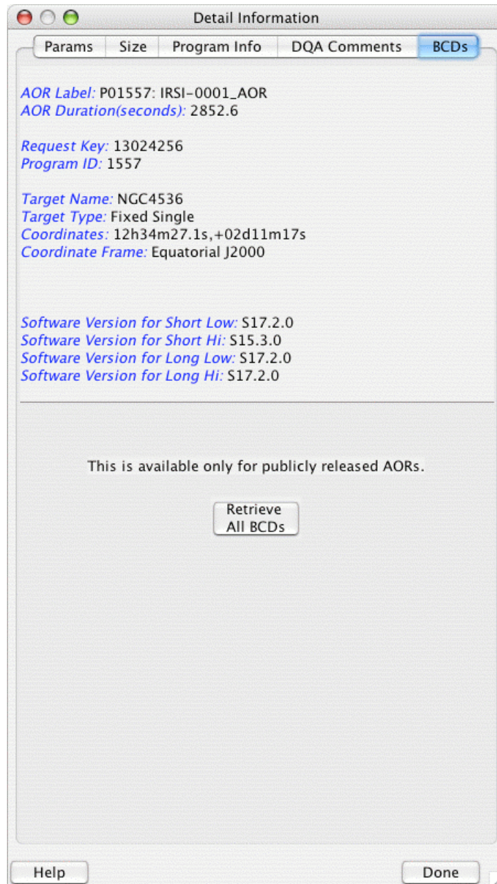
Figure 115: The Detail Information dialog. The BCDs button is highlighted and selected in this dialog. In this example we wish to overlay the BCDs that were produced by this IRS Peak-Up Imaging AOR. You can do this by clicking on the “Retrieve all BCDs” button in the dialog window.
