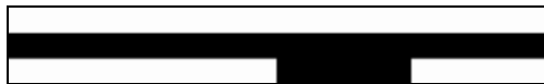
Figure 2.4: Bad pixel mask (pmask) for MIPS-160 data. The center stripe has no detectors (see SOM for details), and the “bite” in the lower right is the inoperative readout.
