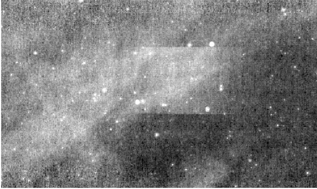
Figure 6.19: Example of single frame with zero-level offset. No background matching was performed in creating this mosaic.
