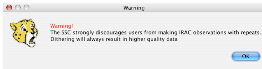
Figure 72: The warning window which now pops up if you select more than one frame per pointing (“repeats”) in all IRAC modes.
