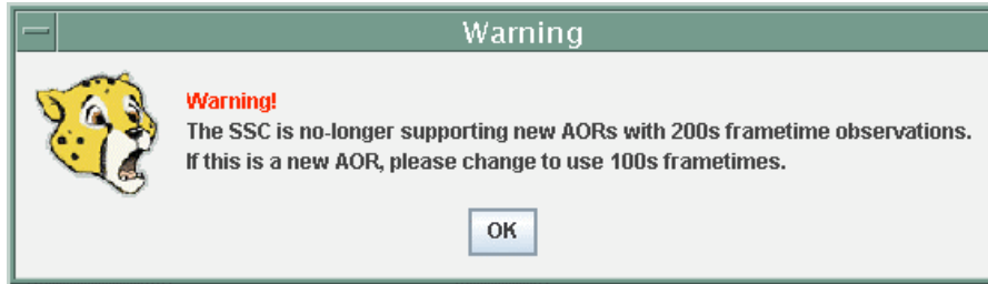
Figure 71: The warning window which now pops up if you select the 200-sec frame time in either IRAC Full Array or HDR modes.
