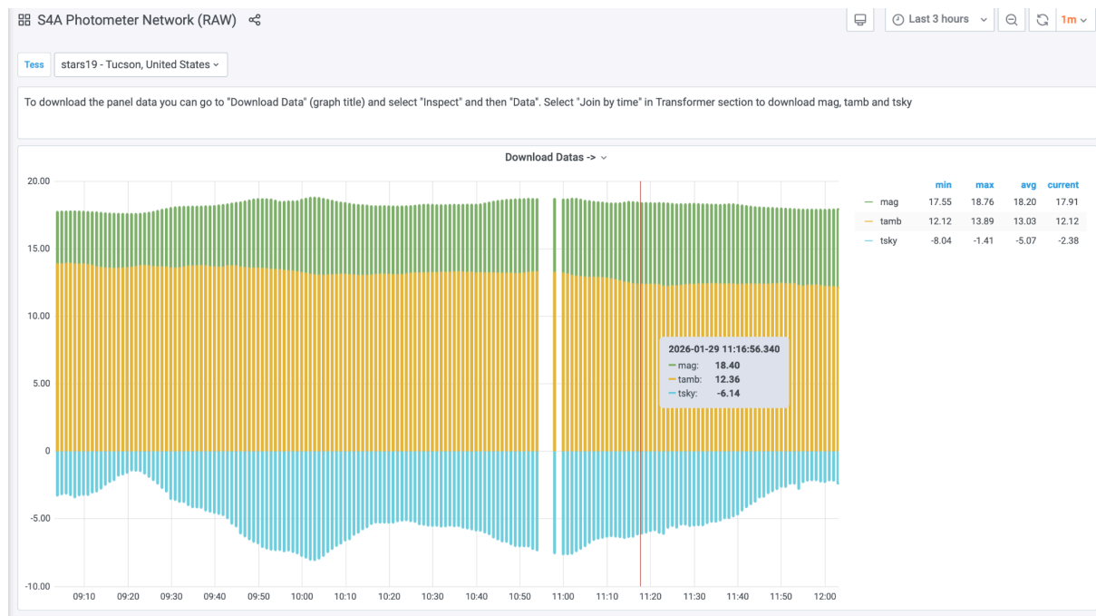
Figure 4. Grafana panel showing raw data arriving to the STARS4ALL repositories in real time. In this example the time range is set to ‘last 3 hours’ but you can change it using the menu at top right.
